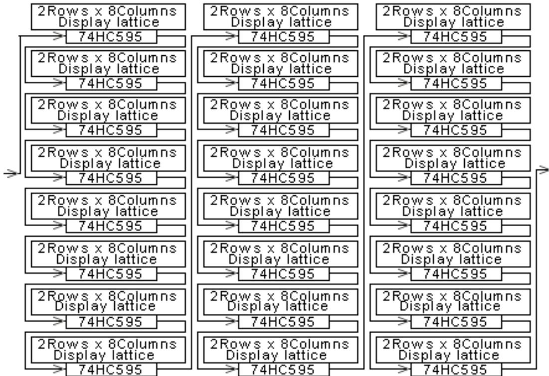
**Mode B: 16 rows/zone:** the signal is shown below; setup method: put the 7<sup>th</sup> switch (1/2) of the receiving card's JP2 on, and keep other switches stay; changing sending card's setup: hardware setup--system setup--row order--reverse per 2 rows, other setups keep default setting.
