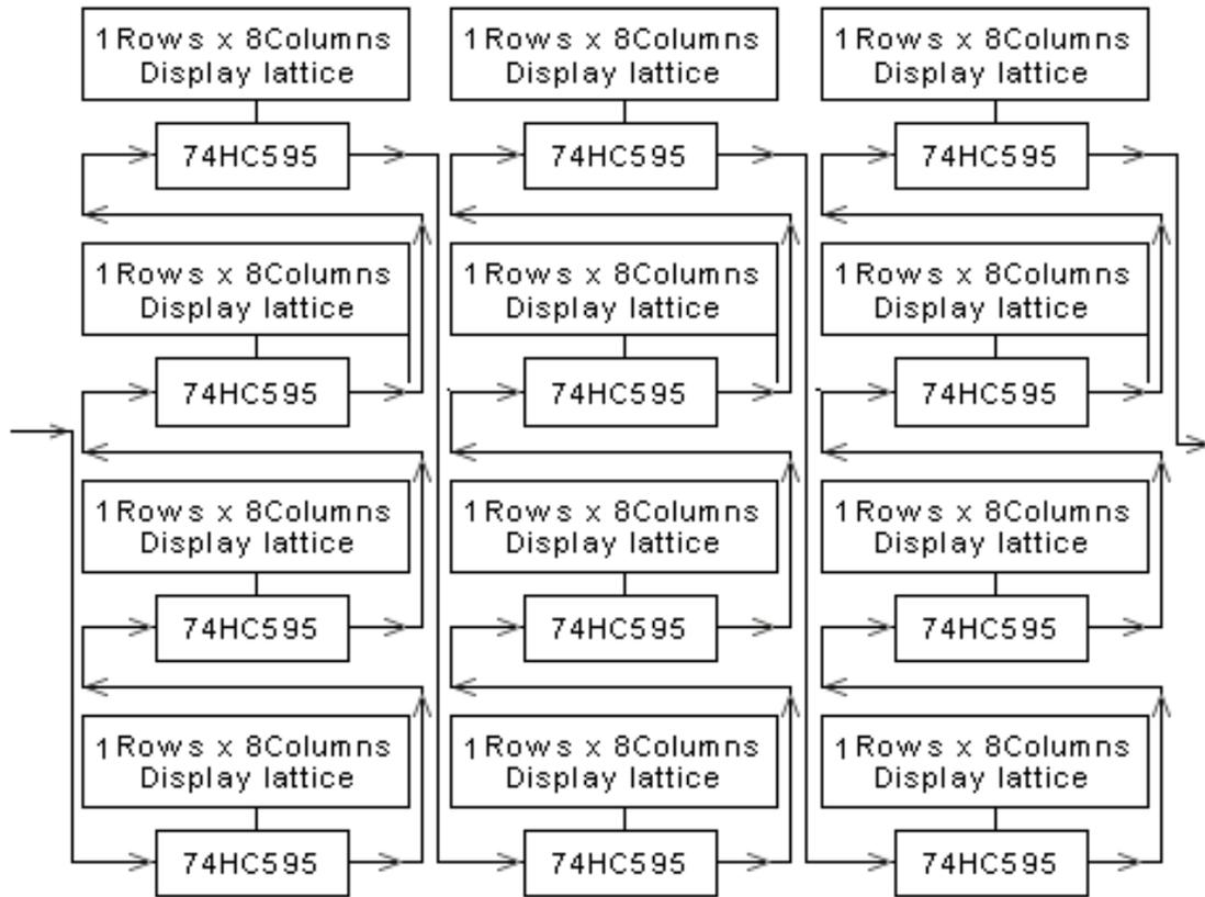
**Mode G 1 row/zone:** the signal is shown below; every receiving card can only drive 1 28 rows height, the maximal display is 512 rows height. The mode can't be setup switch, and it needs to alter program and use special hub card to carry out.
