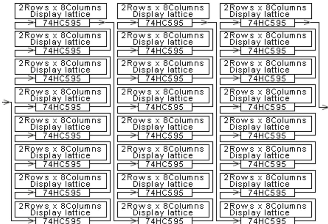
**Mode C: 8 rows/zone:** the signal is shown below; every receiving card can only drive 256 rows height, the maximal display is 1024 rows height; setup method: putting the 7<sup>th</sup>
